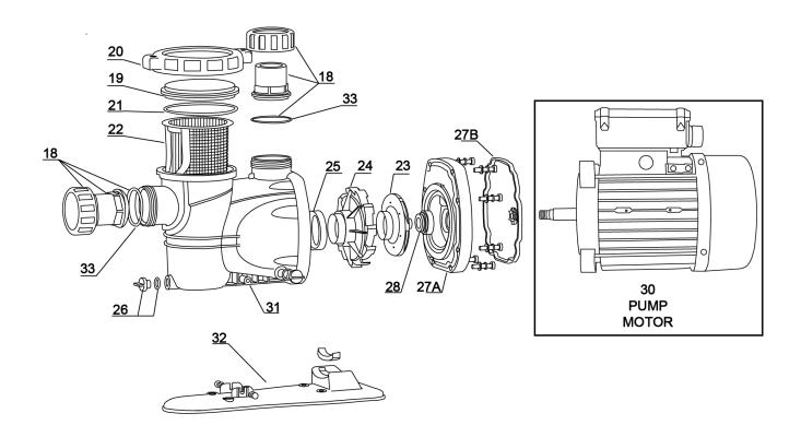
Figure 14 - DV FLO Pump Replacement Parts
