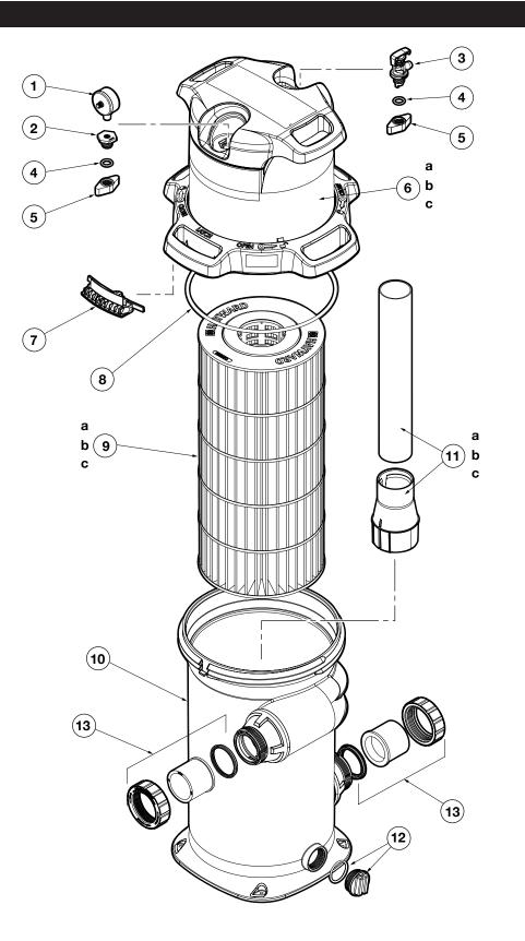
SwimClear<sup>™</sup> C100S, C150S, C200S CARTRIDGE FILTER SERIES REPLACEMENT PARTS
